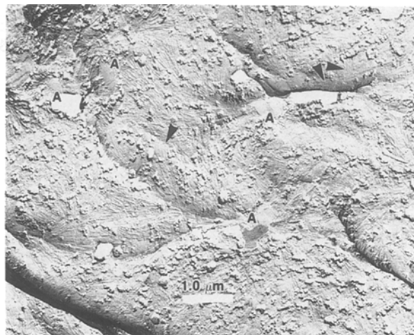
Figure 8 Replica of an etched free surface of melt-crystallized PVF 2 thick film showing lamellae structures. Plate-like structures A, are, suggested to be catalyst residues or additives. Arrows show the areas where the lamellae are lying at a shallow angle to the surface.
